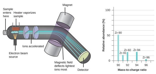
Image credit: Analysis of isotopes in a mass spectrometer by OpenStax Chemistry: Atoms First, CC BY 4.0
